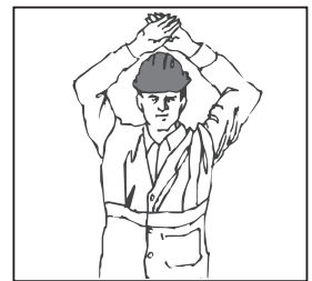
FINISHED WITH CRANE
