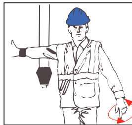
LUFF UP HOIST DOWN
